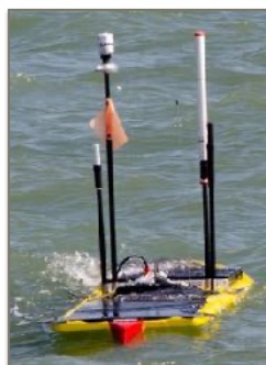
A Liquid Robotics Wave Glider equipped with LOC pH, TA and DIC sensors in the Solent. Photo's courtesy of Socratis Loucaides
