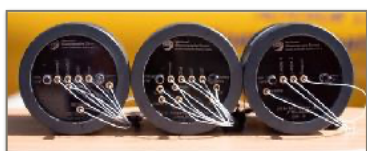
pH, DIC and TA LOC sensors developed through the CarCASS
